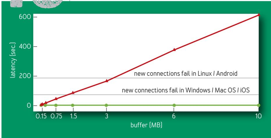
[green] or CUBIC [red] flows. BBR keeps the queue near its minimum, independent of both bottleneck buffer size and number of active flows. CUBIC flows always fill the buffer, so the delay grows linearly with buffer size.
