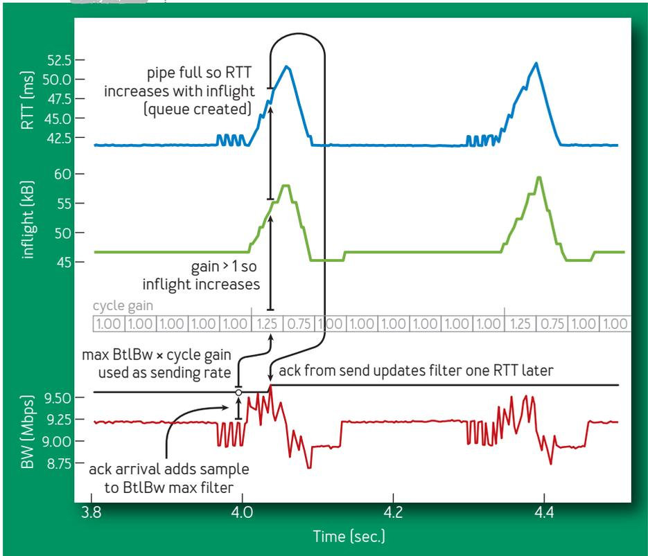
BtlBw has increased, `deliveryRate` increases and the new max immediately increases the BtlBw filter output, increasing the base pacing rate. Thus, BBR converges to the new bottleneck rate exponentially fast. Figure 3 shows the effect on a 10-Mbps, 40-ms flow of BtlBw abruptly doubling to 20 Mbps after 20 seconds of steady operation (top graph) then dropping to 10 Mbps after another 20 seconds of
