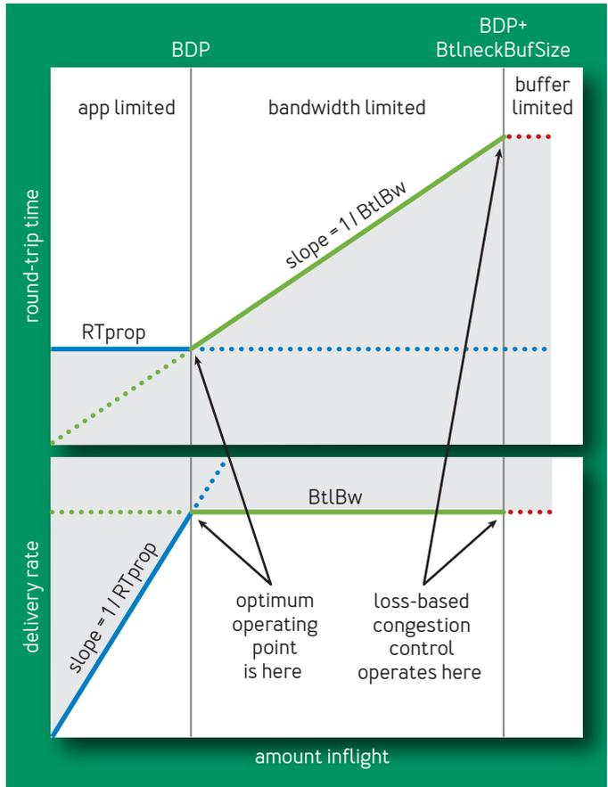
green lines the BtlBw constraint, and red lines the bottleneck buffer. Operation in the shaded regions isn't possible since it would violate at least one constraint. Transitions between constraints result in three different regions (app-limited, bandwidth-limited, and buffer-limited) with qualitatively different behavior.
