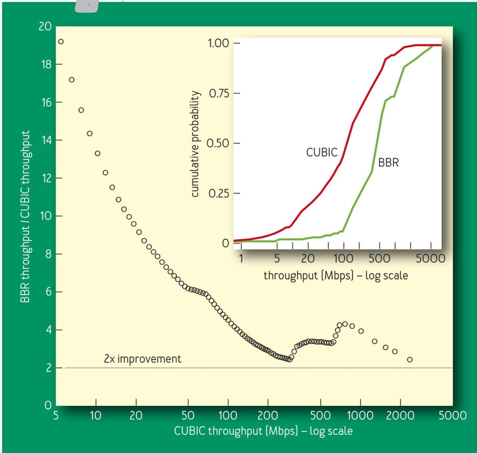
Manually raising the receive buffer on one US-Europe path caused BBR immediately to reach 2 Gbps, while CUBIC remained at 15 Mbps—the 133x relative improvement predicted by Mathis et al.<sup>17</sup>
