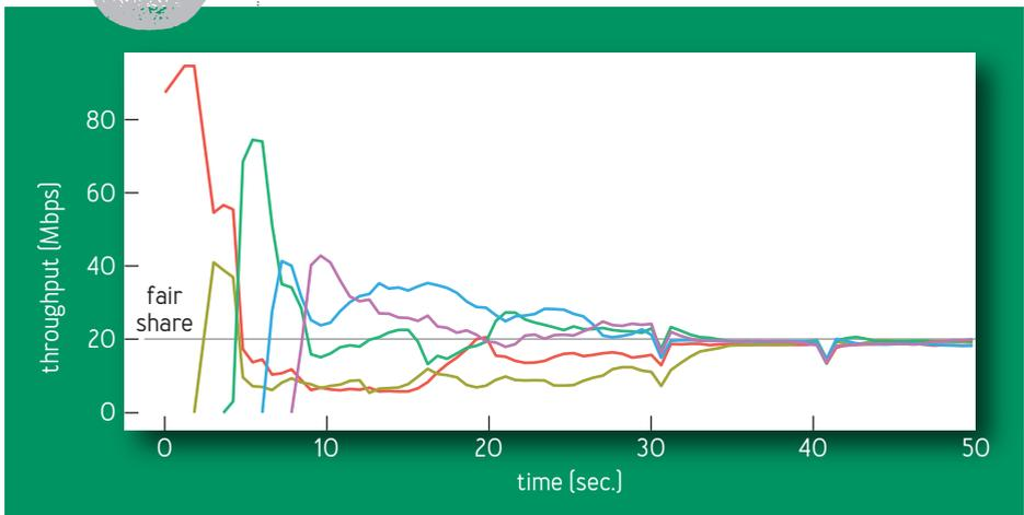
to four packets for at least one round trip, then returns to the previous state. Large flows entering ProbeRTT drain many packets from the queue, so several flows see a new RTprop (new minimum RTT). This makes their RTprop estimates expire at the same time, so they enter ProbeRTT together, which makes the total queue dip larger and causes more flows to see a new RTprop, and so on. This distributed coordination is the key to both fairness and stability.
